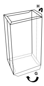
**5** Put tray onto base and lock into tabs as shown.
